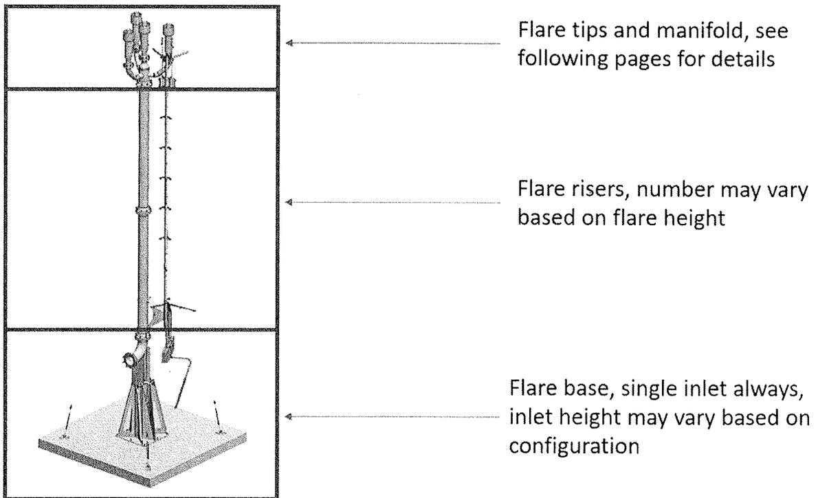
Note: The figures in Appendix A show various multi-tip configurations with the model SHC-6 tip. These configurations can also utilize model SHP-6.
